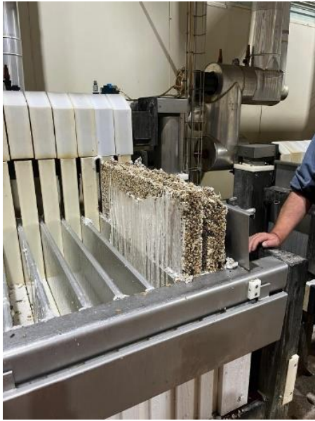
Figures 6 & 7: Block freezer with frozen mussel meat (left) and the packaging (right)
