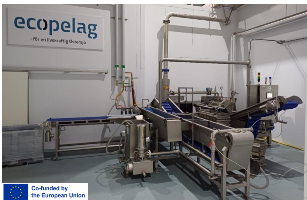
Figure 1: The mussel cooker and meat and shell separation line installed in the processing room at the Baltic Sea factory.
