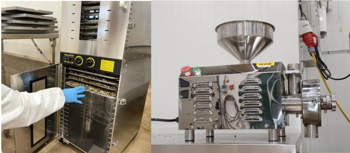
Image 10&11: Mussels in the dehydrator (left). Grinder for pilot-scale mussel meal production (right)
