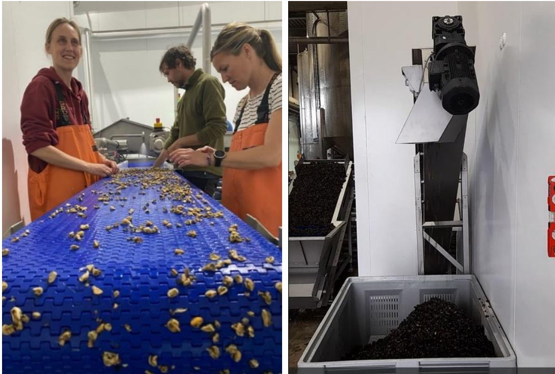
Figures 4 & 5: Separated meat transported on the inspection band (left). The shells are transported with a transport screw out from the process room (right).
