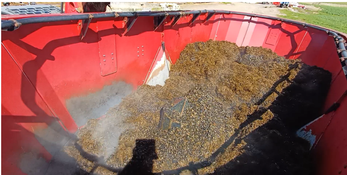
Fig. 8. Picture taken in the beginning of the mixing process when whole mussels could still be seen. The materials emitted heat while mixing.
