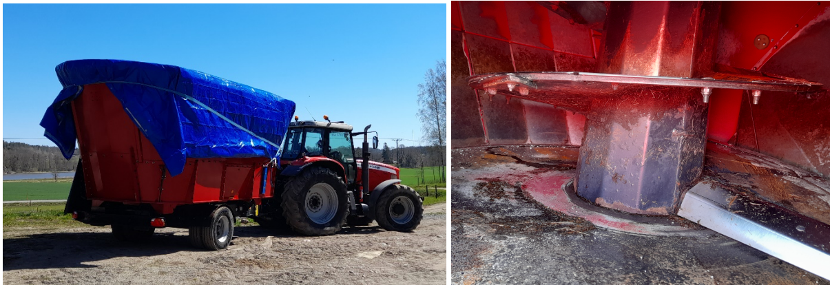
Fig. 3. A feed mixer (this model is Kongskilde VM volume 16 m 3 ) with two internal screws for grinding and mixing. This type of agricultural machines is readily available.
