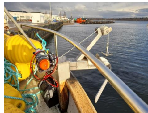
Figure 8: VK26 Garpen. This boat is used for substrate setting, and to mount compensation weights and floats. It can load up to 10 km of substrate rope below deck per journey, and up to 35 buoys on deck in addition to the substrate rope.
