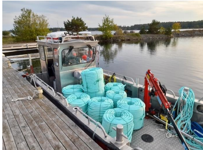
Figure 7 (right): The Ecopelag work boat packed with headlines. This boat is used for assembly of farm parts at sea, substrate setting, precision jobs, general maintenance, monitoring, sampling and smaller repairs.
