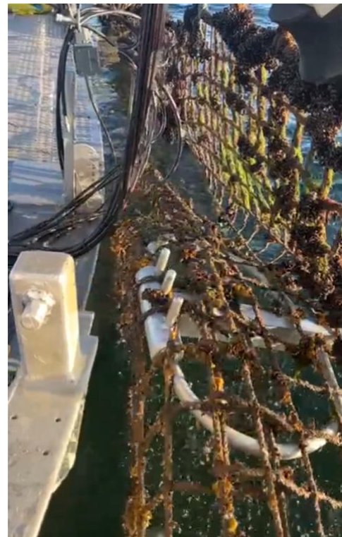
Figure 15: With the development of a hydraulic grab system, the nets are lifted to the boat, and the concrete blocks can be mounted and afterwards gently lowered to the seabed.
