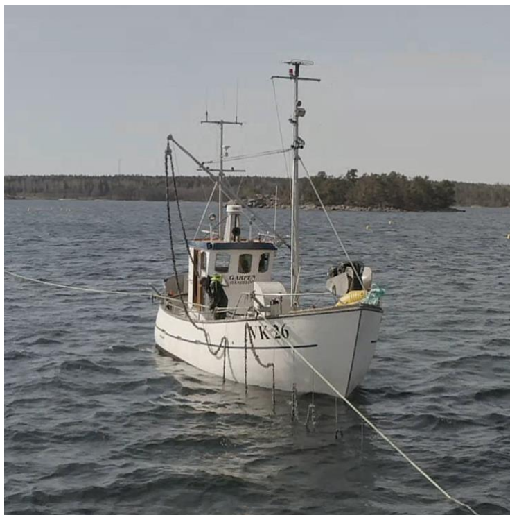
Figure 8: VK26 Garpen. This boat is used for substrate setting, and to mount compensation weights and floats. It can load up to 10 km of substrate rope below deck per journey, and up to 35 buoys on deck in addition to the substrate rope.
