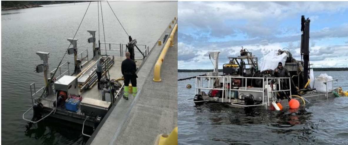
Figure 7: Photos of the new Ecopelag harvester, with capstans and star wheels mounted on an aluminium barge. Left: Freshly delivered from the boatyard. Right: In action. Harvest equipment from Bakker was acquired from the former EU-project Baltic Blue Growth, mounted on the new harvesting pram and complemented with a specially designed mussel sorter/washer.
