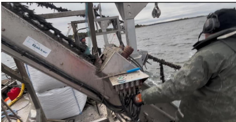
Figure 8: Two people work together on the harvester. Here, one person operates the machinery, and the other person is responsible for cutting loose substrate loops from the headline to feed above an elevator belt where the mussels are continuously scraped off. The scraped substrate rope is then re-attached to the headline, and the mussels pass through the sorter/washer.
