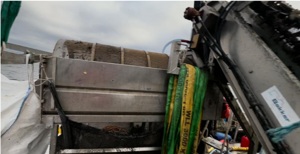
Figure 9: Larger mussels will stay inside the rotating sorter/washer and flush into the collector bag (white), while debris and small mussels are collected in a black net-bag mounted under the sorter.
