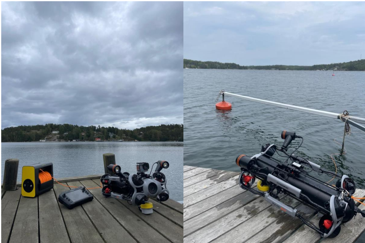
Figure 11: Left: Drone with GoPro camera attached on top, distance sonar lock attached under the drone, and handheld screen with cord E-reel. Right: Drone with laser scaler attached to the top of the drone. Pictures are from a test for mounting and driving the drone in a bay.
